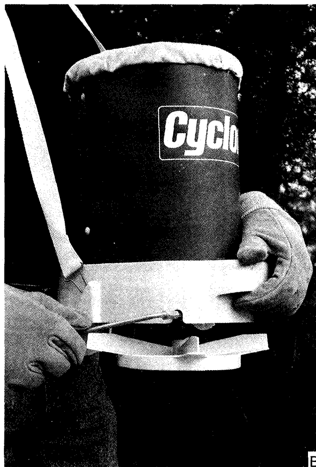
Figure 5.— (A) sack-type and (B) plastic hopper model of hand-cranked spreaders.
