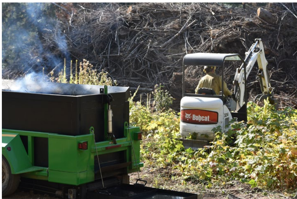
Forest Service scientists, in partnership with Air Burners, Inc., have received a conditional patent to develop a mobile biochar fire box, which turns piles of unmerchantable wood waste into biochar on the spot. USDA Forest Service photo.
