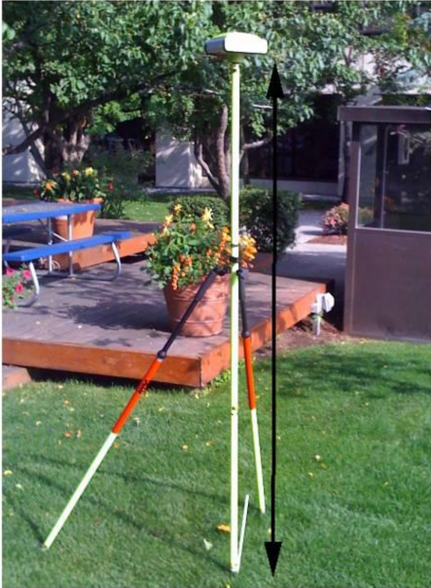
Figure 60. GPS set-up and measurement of antenna height (black line).
