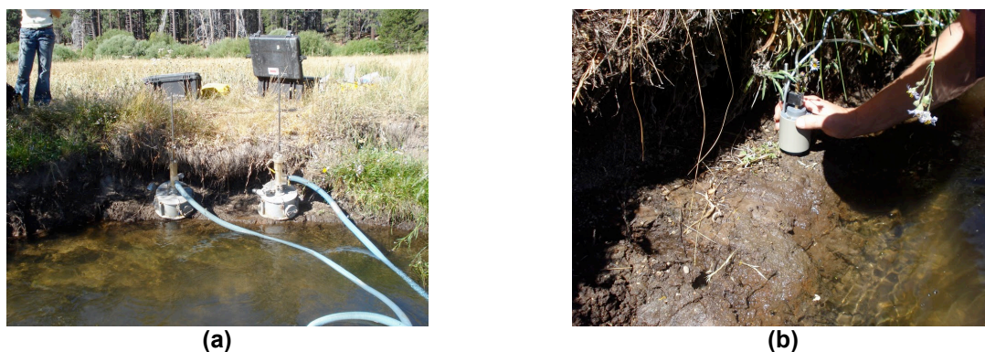
Figure 2 Field instrumentation used in the field campaign of summer 2008 for bank erosion characterization: (a) jet-testing apparatus; (b) Cohesive Strength Meter.
