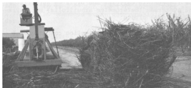
Figure 4--A free standing module, having a density of 8 to 10 lb /ft 3 , ready to be picked up by a transport vehicle.
