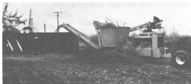
Figure 5--To increase biomass density, the material may first pass through a tub grinder, then into the module builder.
