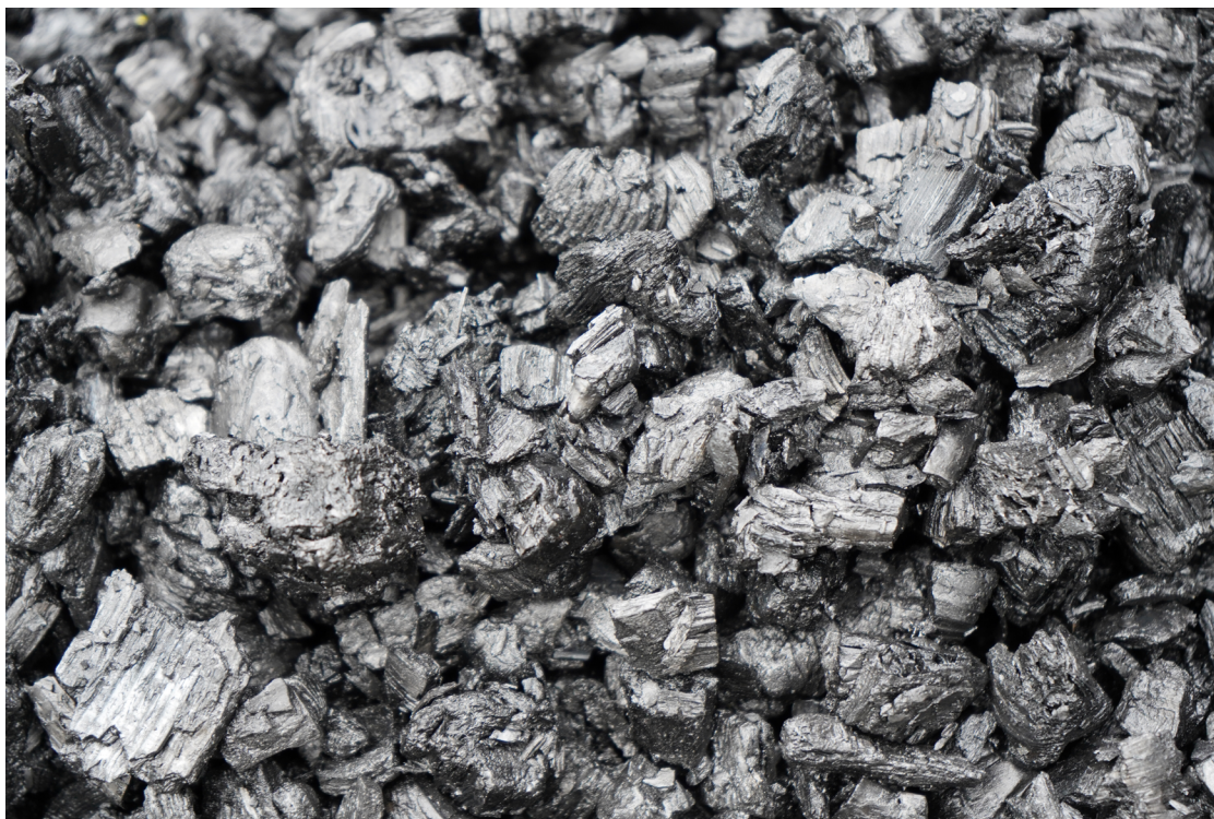
Biochar created from an air curtain burner in Idaho. USDA Forest Service photo by Timothy Nicosia.
