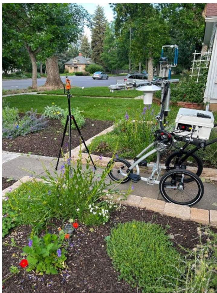
MaRTa outside a home being used to quantify thermal comfort in Fort Collins, Colorado. USDA Forest Service photo.
