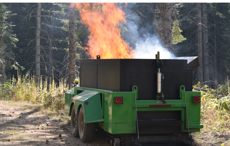
The CharBoss® is an air curtain burner-style mobile biochar production machine. USDA Forest Service photo by D. Weseman.
