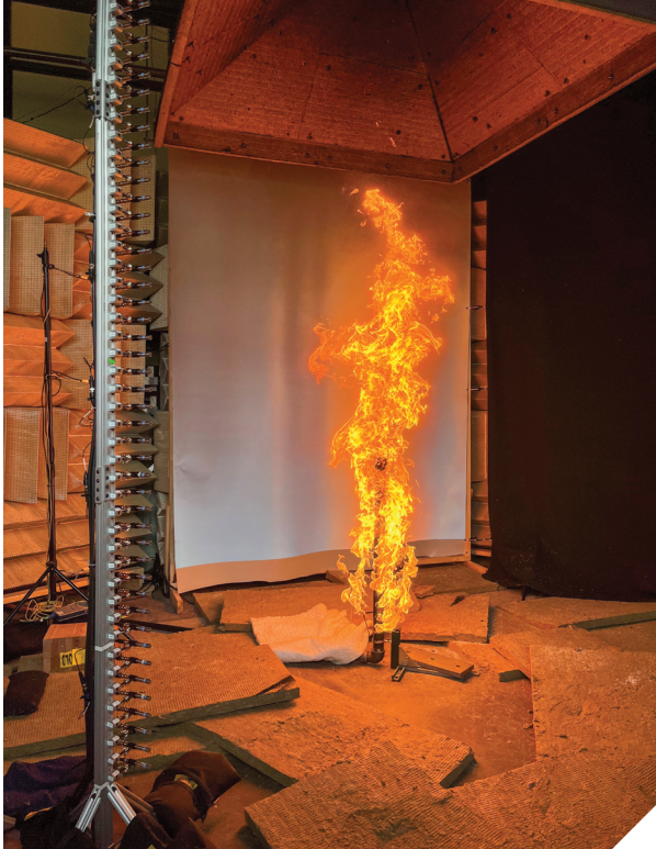
A vertical gas burner and vertical array of microphones used to characterize sound during a non-standard fire measurement study in the fire lab. USDA Forest Service photo by Kara Yedinak
