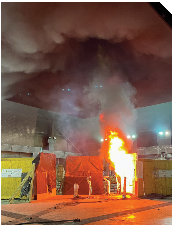
Full-scale structure fire experiments conducted, in part, to investigate emissions and mass timber performance. USDA Forest Service photo by Kara Yedinak.
